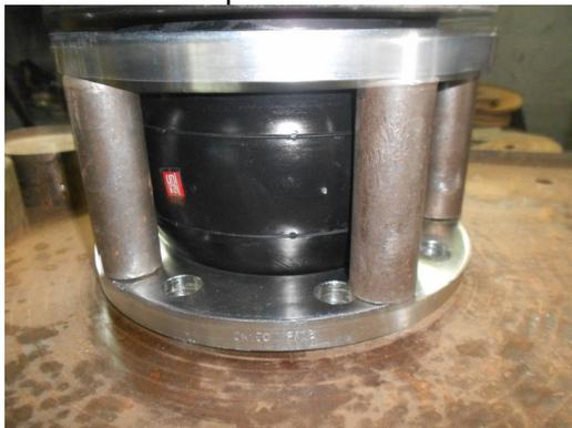
3. Rubber Compensator under pressure
