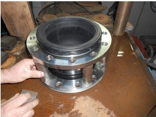
9. Prepare to Hydrostatic Test
