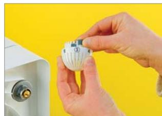
4. Partial closing of the thermostatic head is carried out by inserting the limiter in the cams on the left of the number indicating the min. desired closing (smaller than the initial setting).
