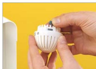
5. In order to fix the ends of the regulation field, up to lock the thermostatic head in the desired setting position, it is necessary to position a limiter on the right of the number indicating the max. desired opening and a limiter on the left of the number indicating the min. desired closing.
